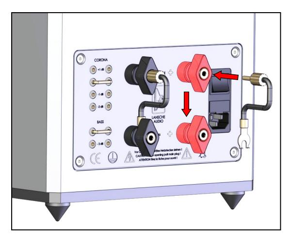
There are 2 cable bridges supplied for each speaker. When using a single wire connection use the bridges as shown on the previous page. This method allows for speaker cables terminated with banana plugs or spade lugs to be used.
